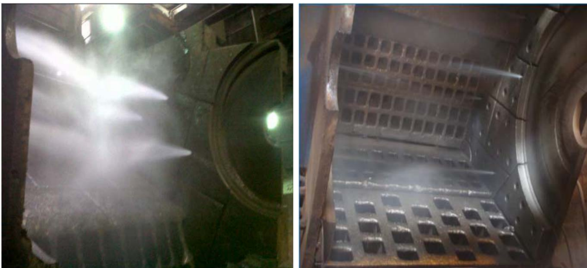
Figure 8: Water spraying in the shredder chamber [9] [10]
